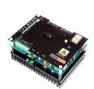
ControllerPart # 3200i/1630/60V AC supply input versionPart # 3200i/16LV60Semiconductor Fuse 14 x 51\*Part # CH00730AFuseholder 14 x 51\*Part # CP102053Pot kit incl graduated dial & knobPart # POTKITFilter (240V operation, if required)Part # FRLN16Filter (415V operation, if required)Part # FRLL16\* Note. Two fuses & holders required for 415V Line to Line operation.
